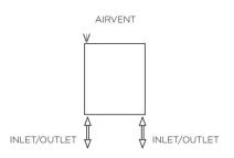
All Dimension are in mm Max.Working Pressure = 10 Bar Max.Working Temprature=95° C Inlet / Outlet: 1/2" BSP
