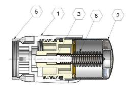
Thermostatic head contains built in sensor (6) filled with liquid of high expansibility. Liquid, located inside of the regulation knob (2) is able to dilate or reduce proportionally to the rise or fall of room temperature, registering even it's slightest variations.
