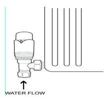
The thermostatic head should be located so that it can constantly sense the temperature of the free air circulating in the room. Try to ensure that the thermostatic head is never conceled behind curtains or closley obstructed by shelving or furniture.
